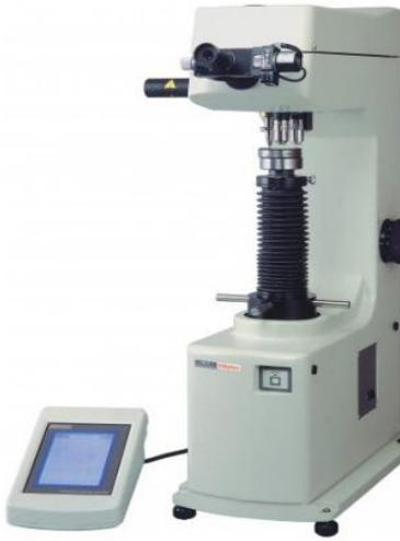
A photograph of a Mitutoyo Hardness Testing Machine HV, Model No. 810-165D. It is a light-colored machine with a vertical frame and a digital control unit at the bottom left. |                                                                                                                                                                                                                                                                            |
